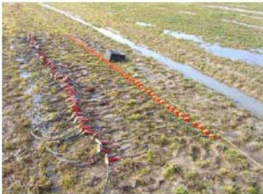
Fig. 3. The photo shows geophones laid out for studying acoustic transmission properties when the ground is water saturated. The experiments were done by Gilcrist. Studies have revealed that the preferred frequency transmission ranges vary somewhat for different types of soil.
