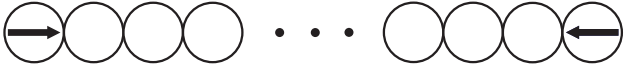
FIG. 1: Schematic setup of a granular chain at initial time. Two incoming pulses of equal velocity start simultaneously at the ends of the chain.
